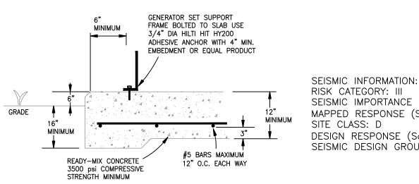
RISK CATEGORY: III SEISMIC IMPORTANCE FACTOR: 1.25 MAPPED RESPONSE (Ss AND S1): 17.2%g & 7.9%g SITE CLASS: D DESIGN RESPONSE (Sds AND Sd1): 18.3%g & 12.7%g SEISMIC DESIGN GROUP: B
