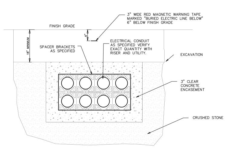
NOTE: DETAIL IS DIAGRAMMATIC ONLY. E.C. TO VERIFY EXACT QUANTITY OF CONDUITS NEEDED WITH ELECTRICAL RISER DIAGRAM AND UTILITY. E.C. TO PROVIDE NEEDED CONDUITS FOR NEW SERVICE AND ONE EXTRA SPARE CONDUIT.
