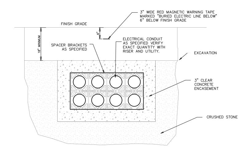
NOTE: DETAIL IS DIAGRAMMATIC ONLY. E.C. TO VERIFY EXACT QUANTITY OF CONDUITS NEEDED WITH ELECTRICAL RISER DIAGRAM AND UTILITY. E.C. TO PROVIDE NEEDED CONDUITS FOR NEW SERVICE AND ONE EXTRA SPARE CONDUIT.
